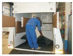
Holding both sides of the mat, pull the mat completely out of the trailer, overlapping the ramp. The trailer can be cleaned, dried out and the mat can be put back into position.
