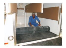
Once the mat is at the back of the trailer you can gain access and clean the floor. Once clean and **dry** the mat can be rolled back.
